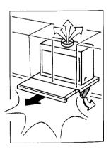
The appliance can be installed to recirculate or extract contaminated air. However, the cooker hood is more effective in the extraction mode.
